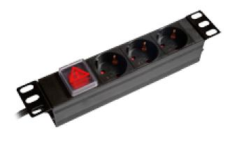
Multiple socket with GER type plug Rack mountable 3 outputs up to 250VAC 16 A max. 1U Integrated on/off switch
